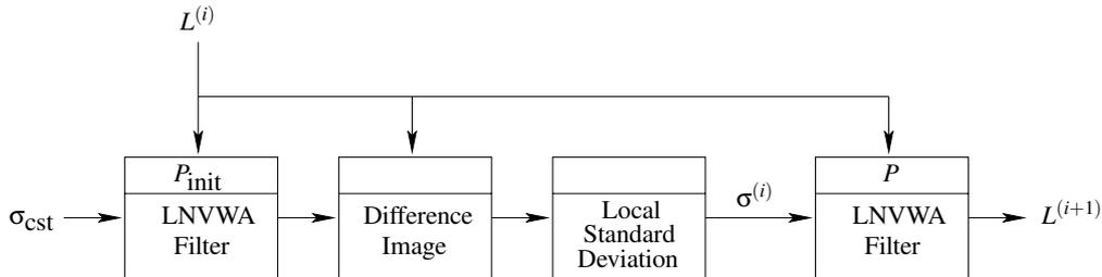
**Figure 3.** Iterative calculation of the noise filtered image  $L^{(i+1)}$  from the previous estimate  $L^{(i)}$ .
