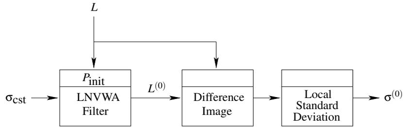
**Figure 2.** The initialization step to determine an initial noise map  $\sigma^{(0)}$  from the input image  $L$  and a uniform noise map  $\sigma_{\text{cst}}$ .
