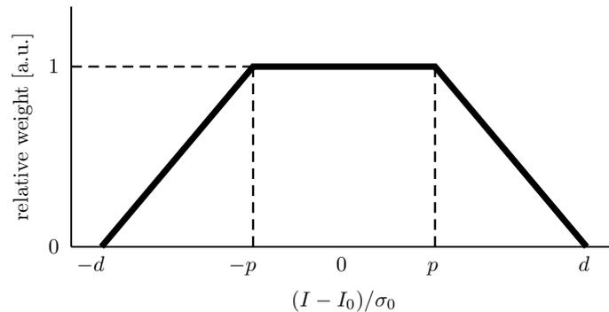
**Figure 1.** The weighting function for the local noise variance weighted averaging filter. The contribution of the intensity  $I$  in a point in the averaging window to the filtered intensity in the central pixel, is determined by the difference between  $I$  and the intensity in the central pixel  $I_0$ , and the standard deviation of the noise at the location of the central pixel  $\sigma_0$ .
